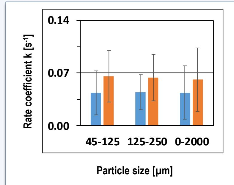
**Carbon conversion** of **plasma** and **thermal** gasification with systematic errors at  $T = 670^\circ\text{C}^{\text{opt,gas}}$
