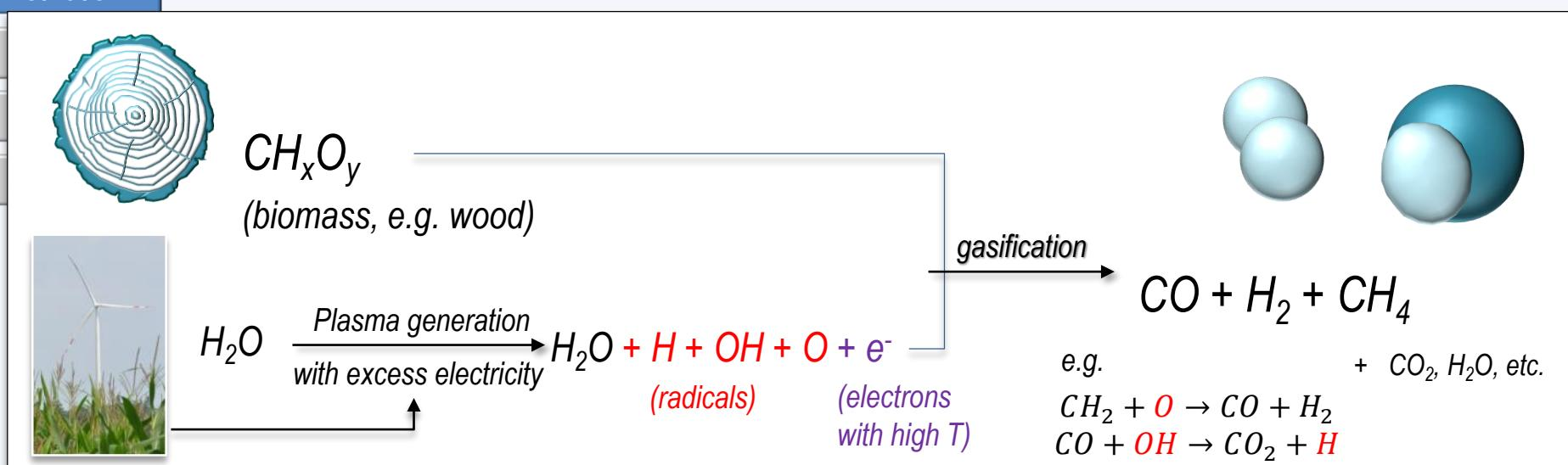
Conventional (thermochemical) biomass gasification with water steam
