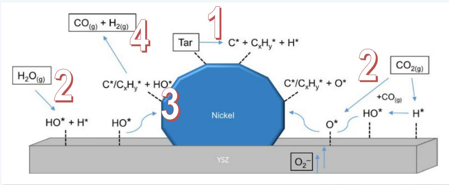
Tar conversion mechanism on SOFC anodes [4]
