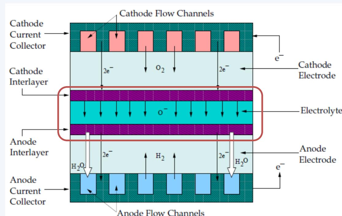
Schematic of a SOFC [5]
