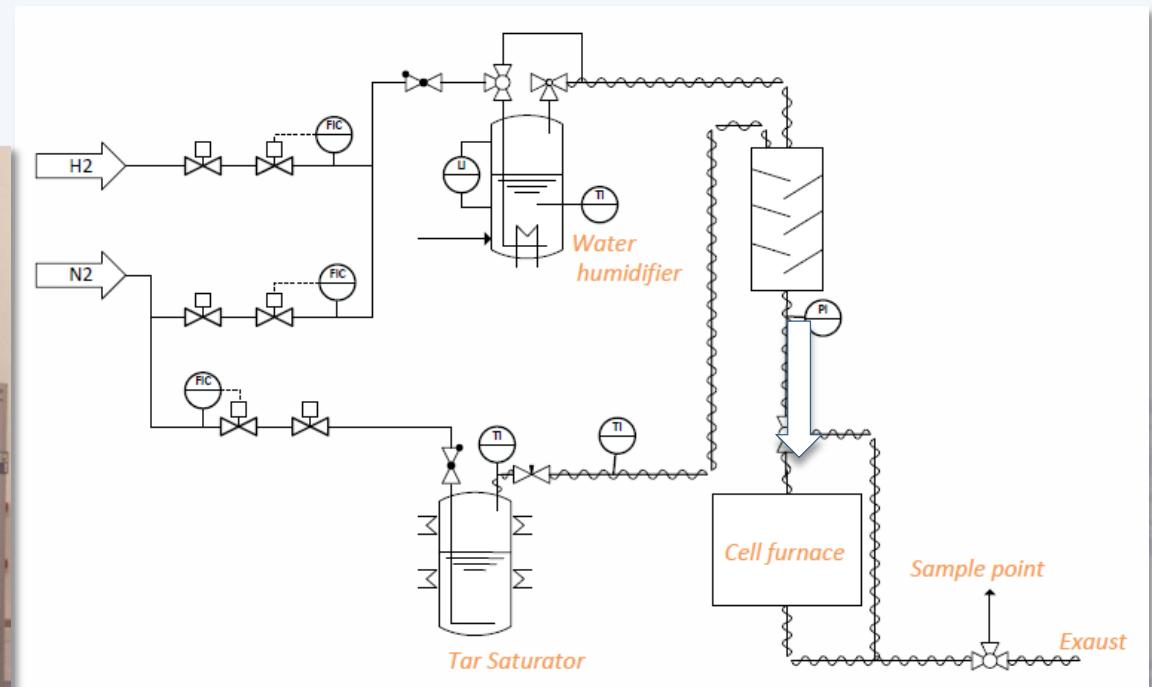
Tar saturator – N<sub>2</sub> as carrier gas saturated with naphthalene
