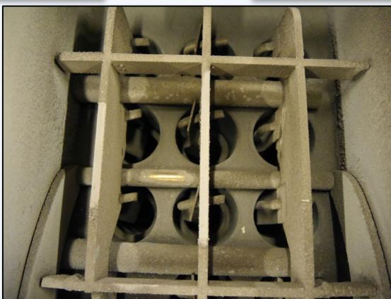
*Condensing flue gas heat exchanger after longterm test*
