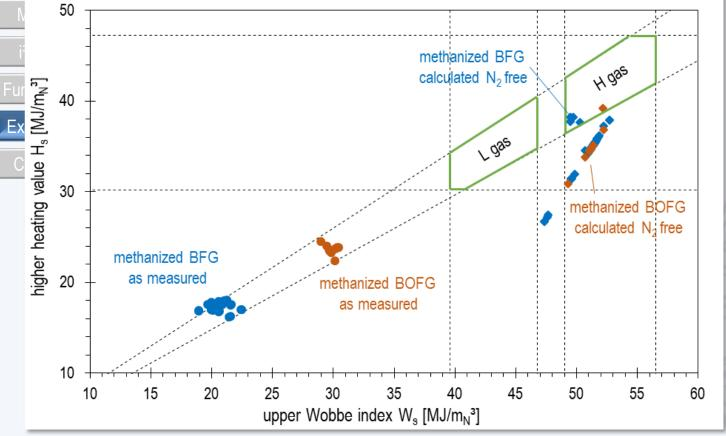
Classification of product gas quality from BFG / BOFG methanation as measured and calculated N2 free (limits according to DVGW G260)
