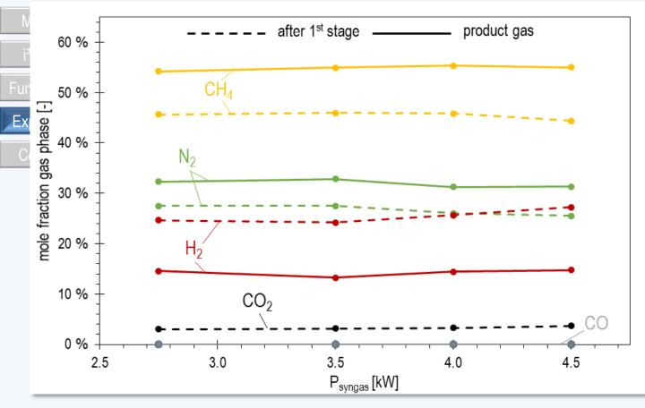
Gas compositions after the 1<sup>st</sup> and 2<sup>nd</sup> methanation stage for different steady-state syngas powers (synthetic BOFG,  $\sigma_{H2}$  = 1.04, p = 4 bar)
