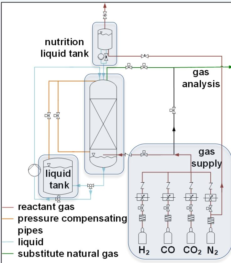
Scheme of the trickle-bed reactor
