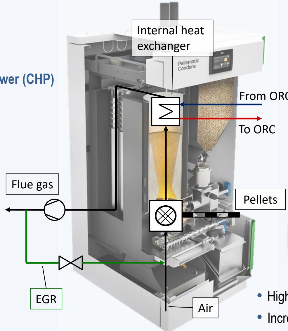
Scheme of an ÖkoFEN pellet boiler with internal heat exchanger and exhaust gas recirculation
