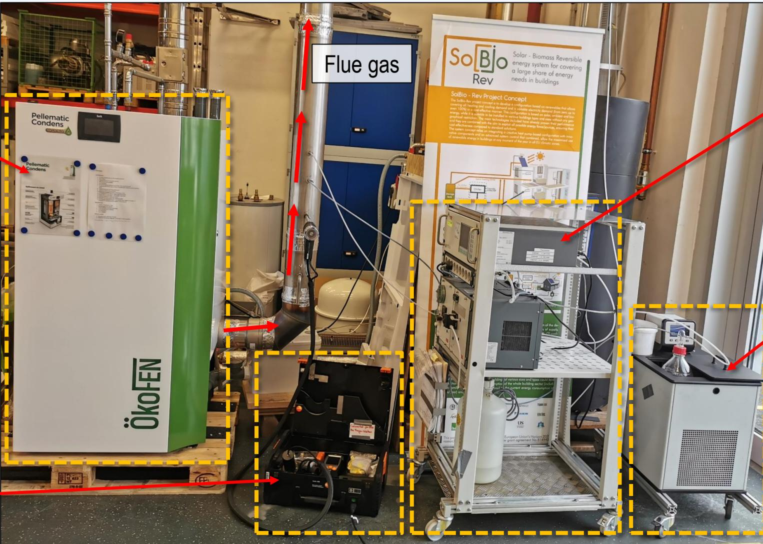
Set-up of the pellet boiler with the flue gas analyzers in the EVT lab
