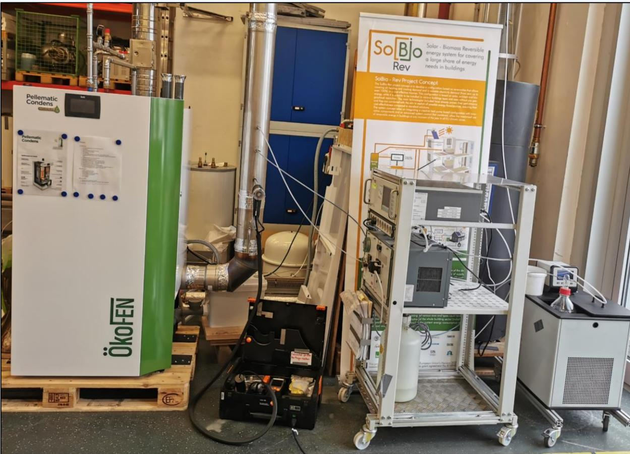
Folie 3 Set-up of the pellet boiler with the flue gas analyzers in the EVT lab
