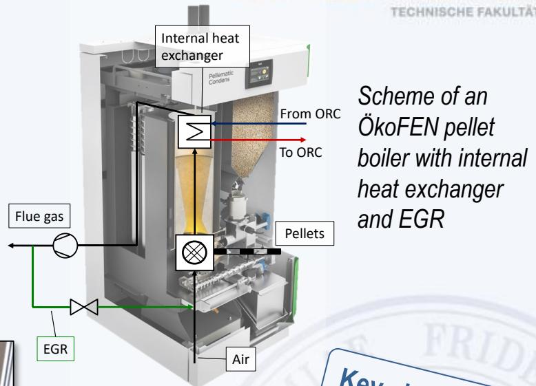
Scheme of an Ökofen pellet boiler with internal heat exchanger and EGR
