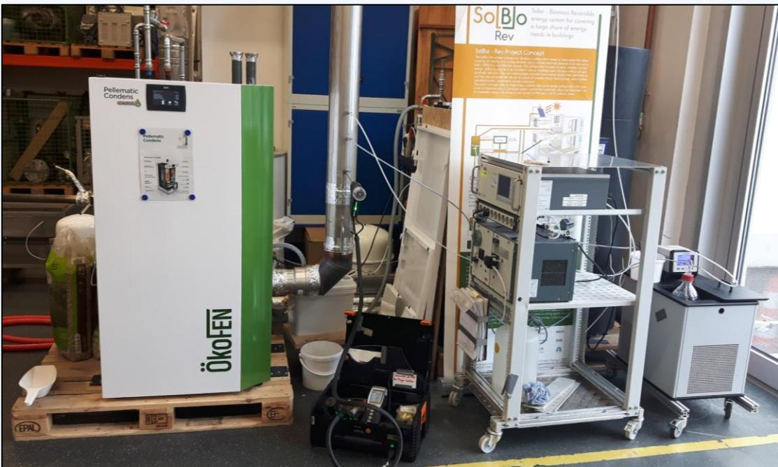
Set-up of the pellet boiler with the flue gas analyzers in the EVT lab
